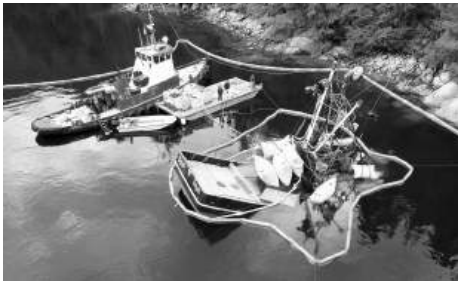
A seiner being raised from 60' by Hanson Maritime in Crawfish Inlet, south of Sitka, 2020. "We were able to boom the wreck, remove over 3,000 gallons of fuel, and remove the vessel in a controlled, quick manner that prevented the closure of the fishing area for the season," says Hanson. (Photo by Rafe Hanson)
