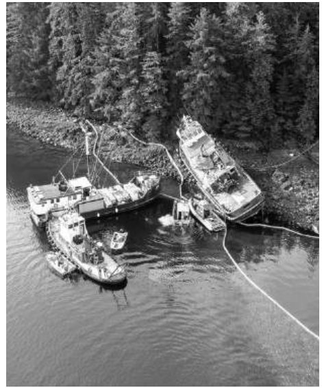
Hanson Maritime tugboat "Salvation" is shown with the "Eyak" which, with tanks on deck, helped transport some of the 43,000 gallons of diesel lightered from the vessel or recovered from containment boom. 2022. (Photo by Rafe Hanson)
